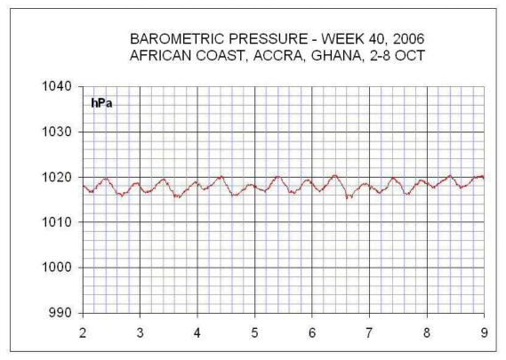
**Figure 7:** When in the tropics systematic pressure variations with a period of close to 12 hours were observed. Note how every second wave top appears slightly smaller than the one before it.
