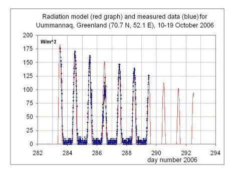
**Figure 4:** The data shown in this figure were collected by Simme Eriksen using a Sol-Data 80spc pyranometer. The red graph shows the model calculation for this very northern latitude. Typically for pristine Arctic locations, a value of the attenuation factor a = 0.85yielded the best agreement with the data. Notice how the solar irradiance is decreasing day by day as the total darkness of the coming Arctic winter draws closer in late October.
