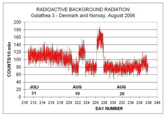
**Figure 5:** At sea the radioactive background radiation remained nearly constant around 80 counts every 10 minutes. Near coastlines or in port the background radiation would sometimes increase dramatically. The two peaks observed in this figure are from Amalie Quay in Copenhagen, Denmark, and from dry dock in Stavanger, Norway.
