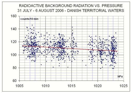
**Figure 6:** *While in port these data were recorded showing the correlation between the radioactive background radiation and the atmospheric pressure.*
