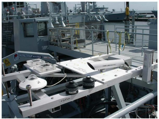
**Figure 2:** The optics table was an aluminum frame firmly fastened to the aft port side of the vessel near the rail. The sky luminance sensor (at right) points towards the horizon with an elevation angle of about 10 degrees. The two SolData photovoltaic pyranometers are visible at the left rear behind the Kipp-Zonen CM 11. In the foreground are a UVB detector and a lux detector. The Geiger-Müller detector at the right measured ionizing radiation.
